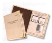
Used to verify the accuracy and calibration of magnetic or eddy current-type coating thickness gages. Includes a zero (uncoated) plate and two other coated plates of certified thickness mounted in a durable leatherette case. Certificate of Accuracy included. Directly traceable to the N.I.S.T. Available in ferrous or Non-Ferrous as follows:
